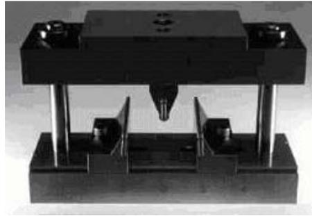
Figure 2: Three-point bending (short-beam) test fixture
