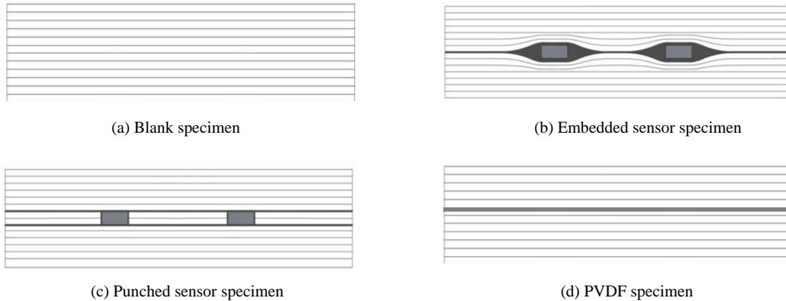
Figure 1: Specimen configurations
