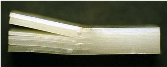
Figure 3: Blank fatigue specimen.
