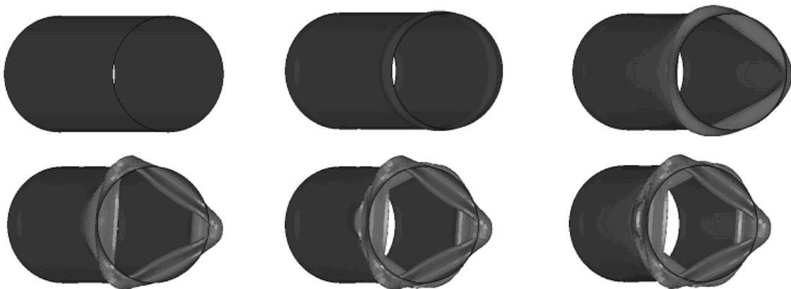
**Fig. 2.** Simulation steps of aluminum tube buckling in uniaxial compression; displacement-controlled loading with crosshead speed  $6.71 \times 10^{-3}$  mm/s.
