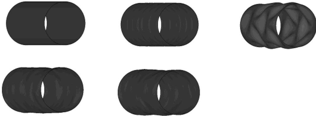
**Fig. 1.** Finite element simulation of the thin NiTi tube buckling, followed by the recovery and permanent deformations; ratio of L/D is 2.5.
