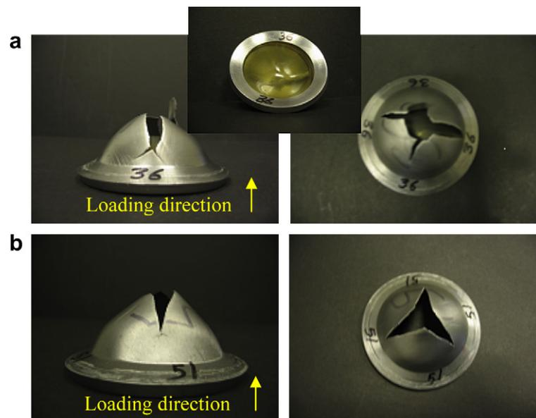
Fig. 8. Deformed steel-plate sample loaded on the dish side at approximately the same kinetic energy per unit thickness: (a) SP-36: bilayer plate loaded on the polyurea side; and (b) S-51: monolithic steel plate.
