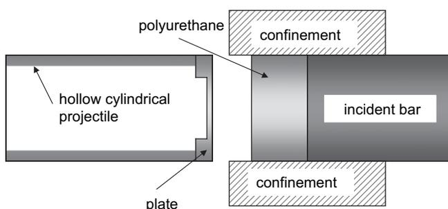
Fig. 1. Schematic view of the reverse ballistic experimental setup.
