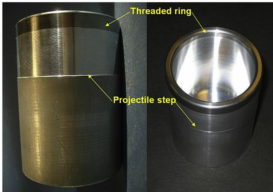
Fig. 4. Projectile used in *set-II* experiments, comprised of a stepped 7075 aluminum tube and a threaded steel ring (left: side view; right: angled view).
