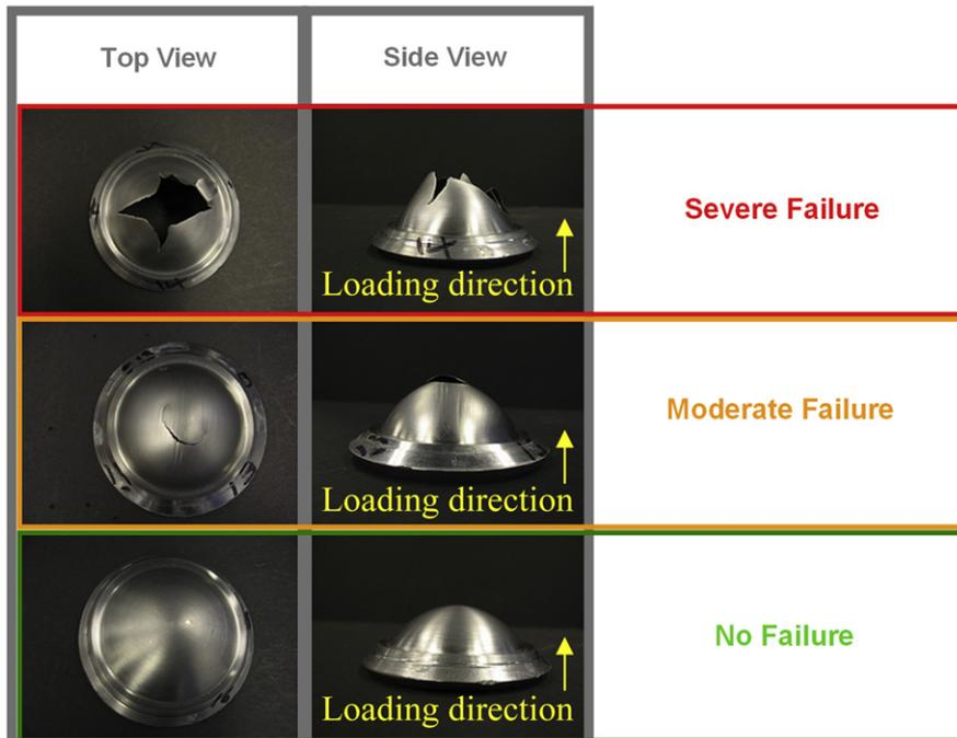
Fig. 6. Side view (right column) and top view (left column) of selected sample for each category of deformed steel plates: severely failed, moderately failed, and not failed.
