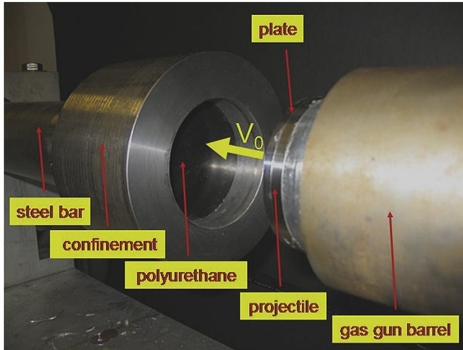
Fig. 5. Experimental setup. The projectile carrying the steel plate is propelled by a gas gun at a controlled velocity towards the confined polyurethane target that rests against a 3-inch steel bar.
