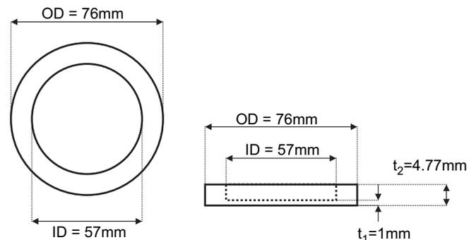
Fig. 2. Schematic view of monolithic steel plate: geometry and dimensions.
