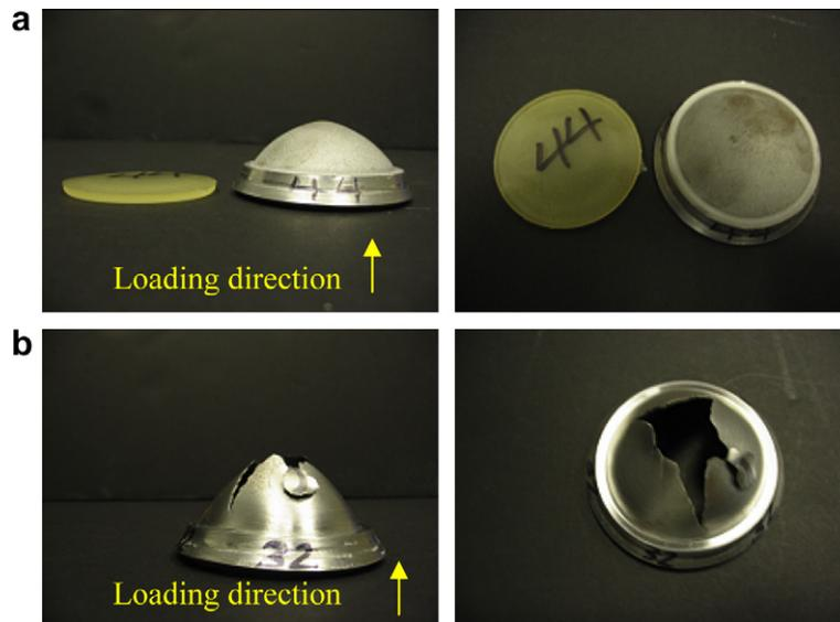
Fig. 7. Deformed steel-plate samples loaded on their flat side at approximately the same kinetic energy per unit thickness: (a) SP-44: bilayer plate loaded on steel side; and (b) S-51: monolithic steel plate.
