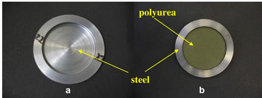
Fig. 3. Un-deformed steel plates: (a) without polyurea coating (left side); (b) with polyurea coating (right side).
